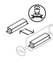
Operating device replaceable by electrician
